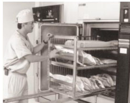
Oxyfume 2002 is used in large chambers. Large devices and trays are more easily processed.
