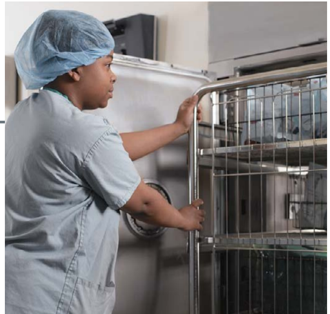
Oxyfume 2000 is used in large chambers, such as this 30 cubic foot hospital sterilizer, in which large devices and trays are more easily processed.
